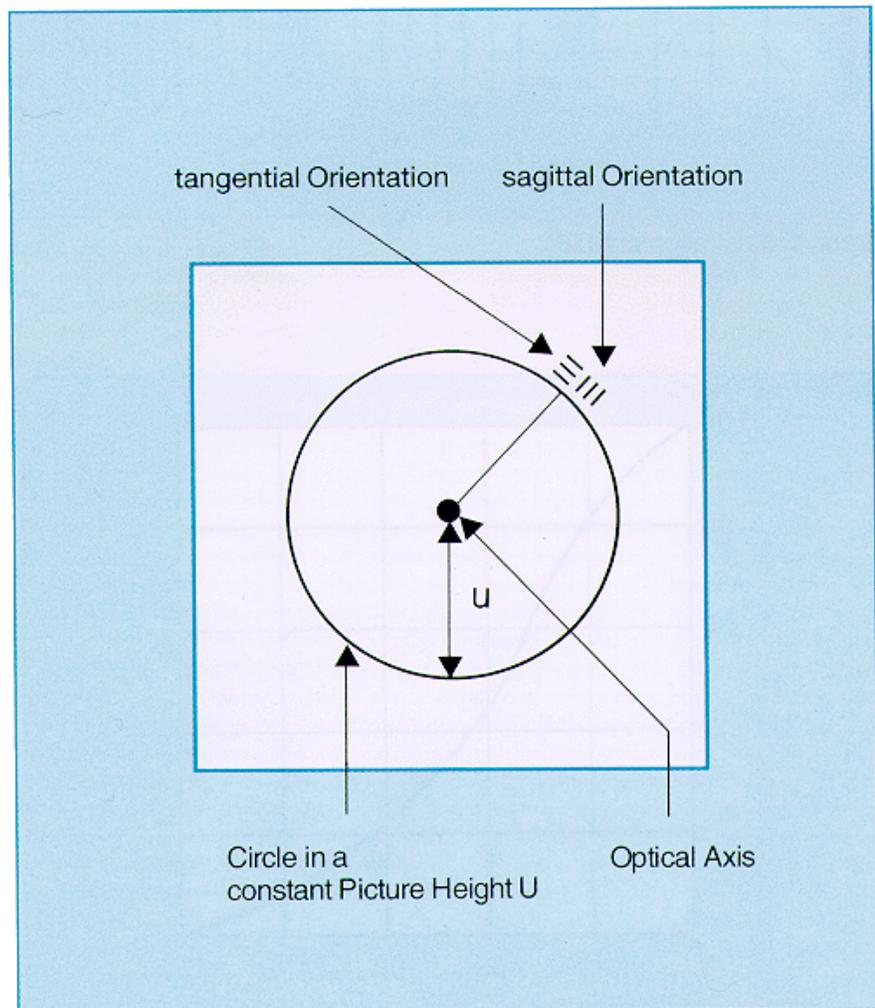
Graph 3: Illustration of sagittal and tangential test frequencies. (Referring to DIN 58185 in Illustrations of MTF data sheets the relation of Object-/Image size is called  $u/u'$ )
